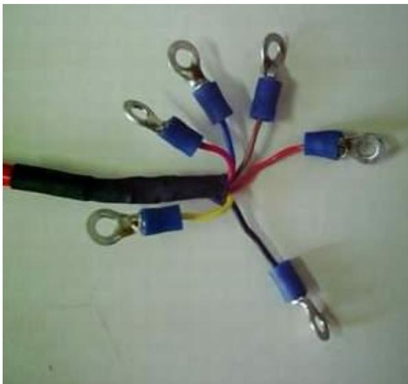
Image: RJ-45 cable with 5 Dry-contact wires
