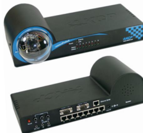
Live full-color streaming video is available at up to 15 fps on a local network via the web interface. Standard JPG format pictures are used allowing the use of third party host tools to store and analyze the JPG pictures. The pictures can be easily downloaded from the CameraProbe8 into the local host where standard software can be used.
